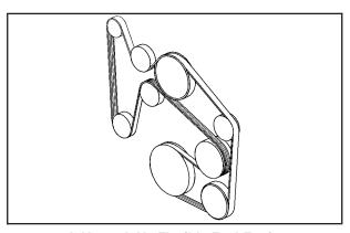
3.5L V6, 3.5L V6 Flexible Fuel Engines, and 3.9 V6 Engines
